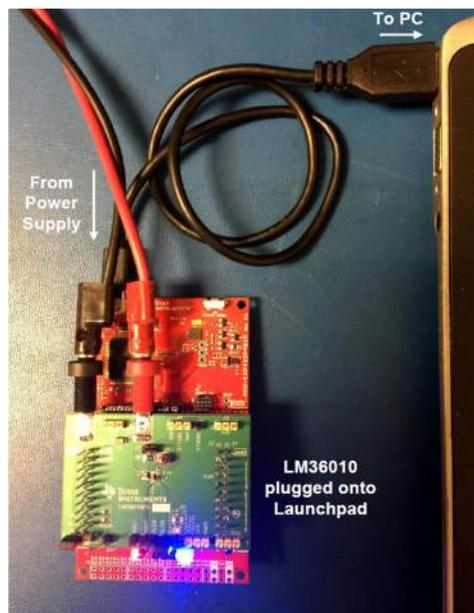
**Figure 6. LM36010EVM Test Setup**
