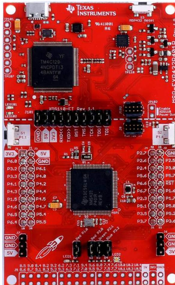
Driver XDS110 of the MSP432 LaunchPad must be installed to use the Texas Instruments LM36010 GUI. Go to [XDS Emulation Software Package](#) to download the driver. On the driver download website, click “3 XDS110 Reset Download” under Contents.
